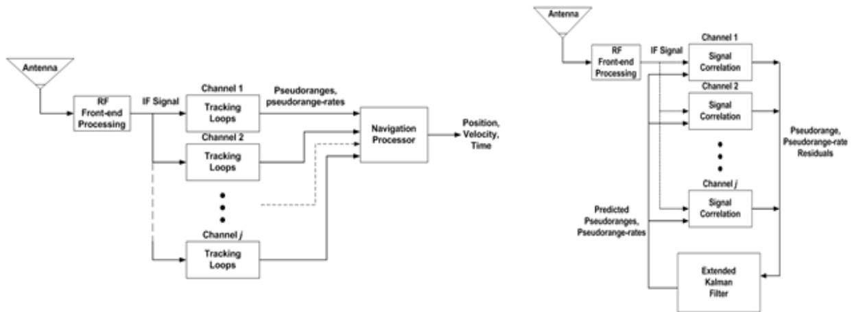
**Figure ES-1. [Left] Standard, Scalar GPS Tracking Loop Architecture [Right] Vector Tracking GPS Receiver Architecture**
