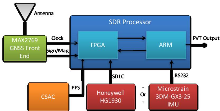
**Figure ES-3. Block Diagram of Hardware Components for the VTRx Receiver.**
