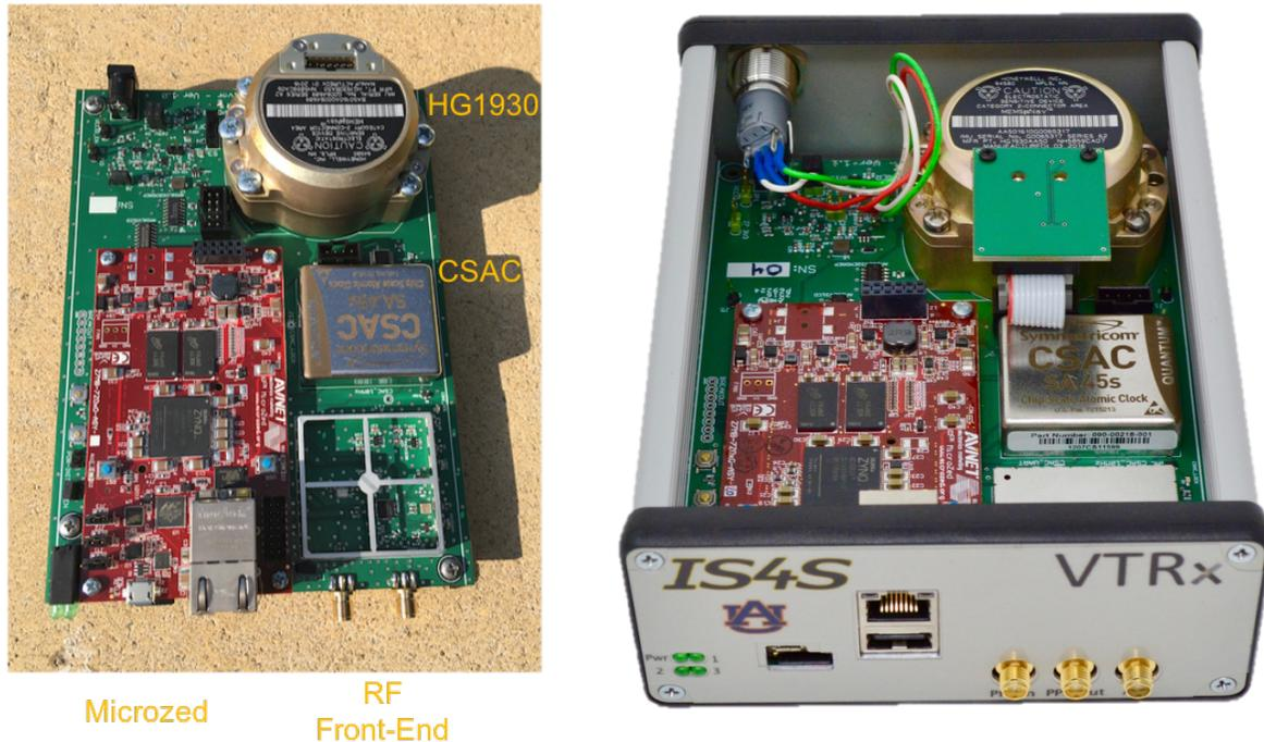
**Figure ES-4. Final Prototype Hardware**
