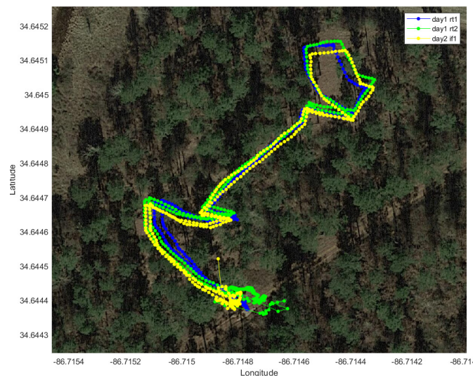
Figure 7-37 Point Map Showing Repeatability of the Vector Tracking Receiver Position Solution at Site 13
