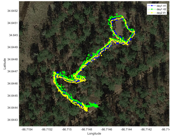
Figure 7-36. Point Map Showing Repeatability of the Novatel Receiver Position Solution at Site 13
