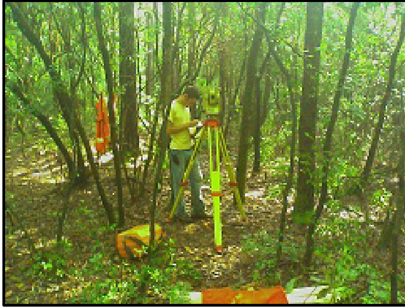
Figure 1-2. Surveyor Operating a Robotic Total Station
