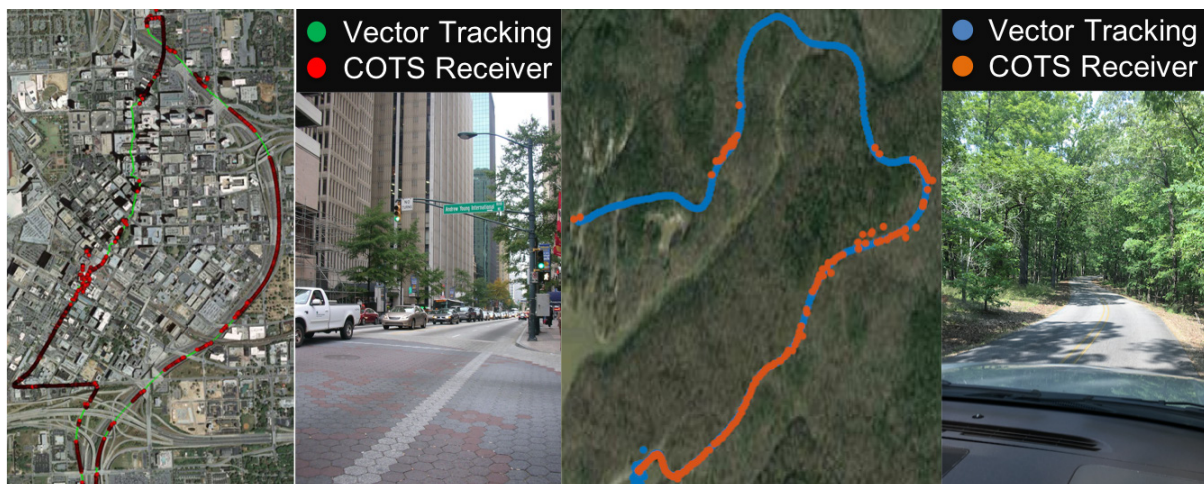
Figure 2-21. Plots of the Vector Tracking Position Solution Compared to a COTS GPS Receiver in Urban and Heavy Foliage Environments Showing the Improved Performance of the Vector Receiver.
