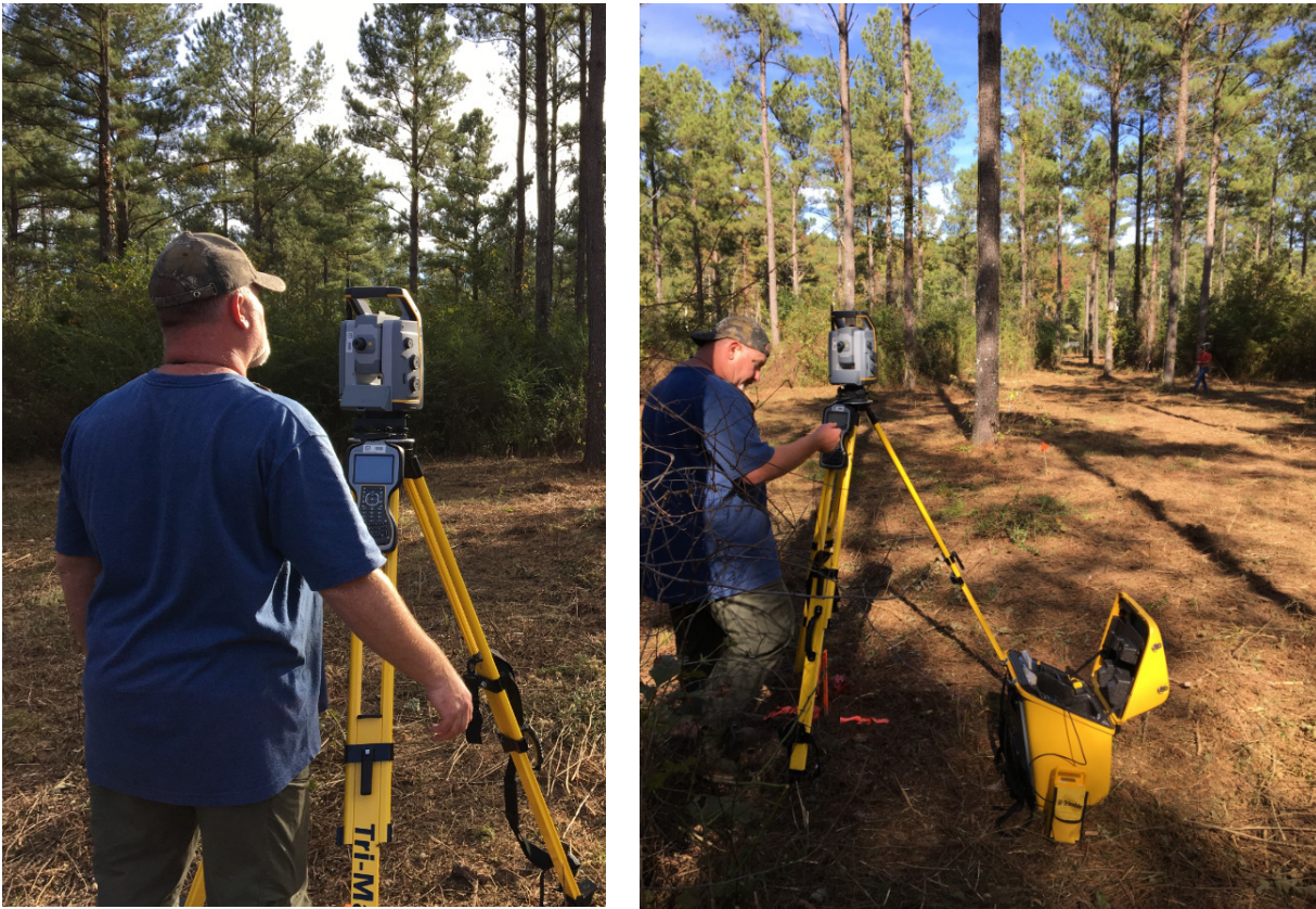
Figure 5-7. Trimble IS System Including Trimble Controller / Data Logger and Trimble VX Total Station
