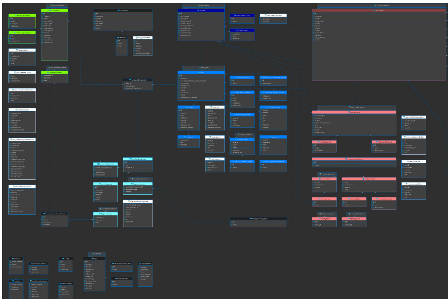
Figure 12. Entity Relationship Diagram (ERD) of the DIMSpec relational database (SQLite) schema demonstrating modularity by collecting tables and view into conceptually related nodes. Individual nodes share a color and visual proximity. Tables are colored, and related views are in white. Details may be difficult to see in this medium, and interested parties are directed to descriptions and higher resolution images of the individual nodes in the User Guide ( https://pages.nist.gov/dimspec/docs/technical-details.html#database-schema ), or the full resolution version hosted in GitHub at ( https://raw.githubusercontent.com/usnistgov/dimspec/refs/heads/main/dimspec_user_guide/assets/ERD.png ).
