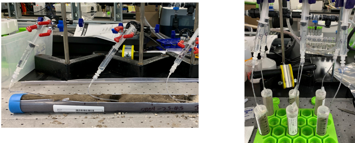
Figure 5-1. Bench-scale Porewater Sampling Using the Micro-sampling Lysimeters.
