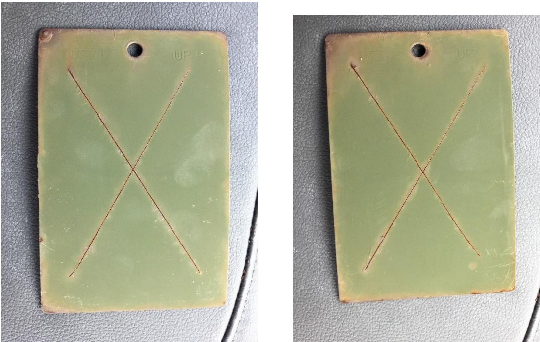
Figure 102. SILSBOND Pretreatment 01 (2%) + Primer + Topcoat on blasted CRS at 24 months
