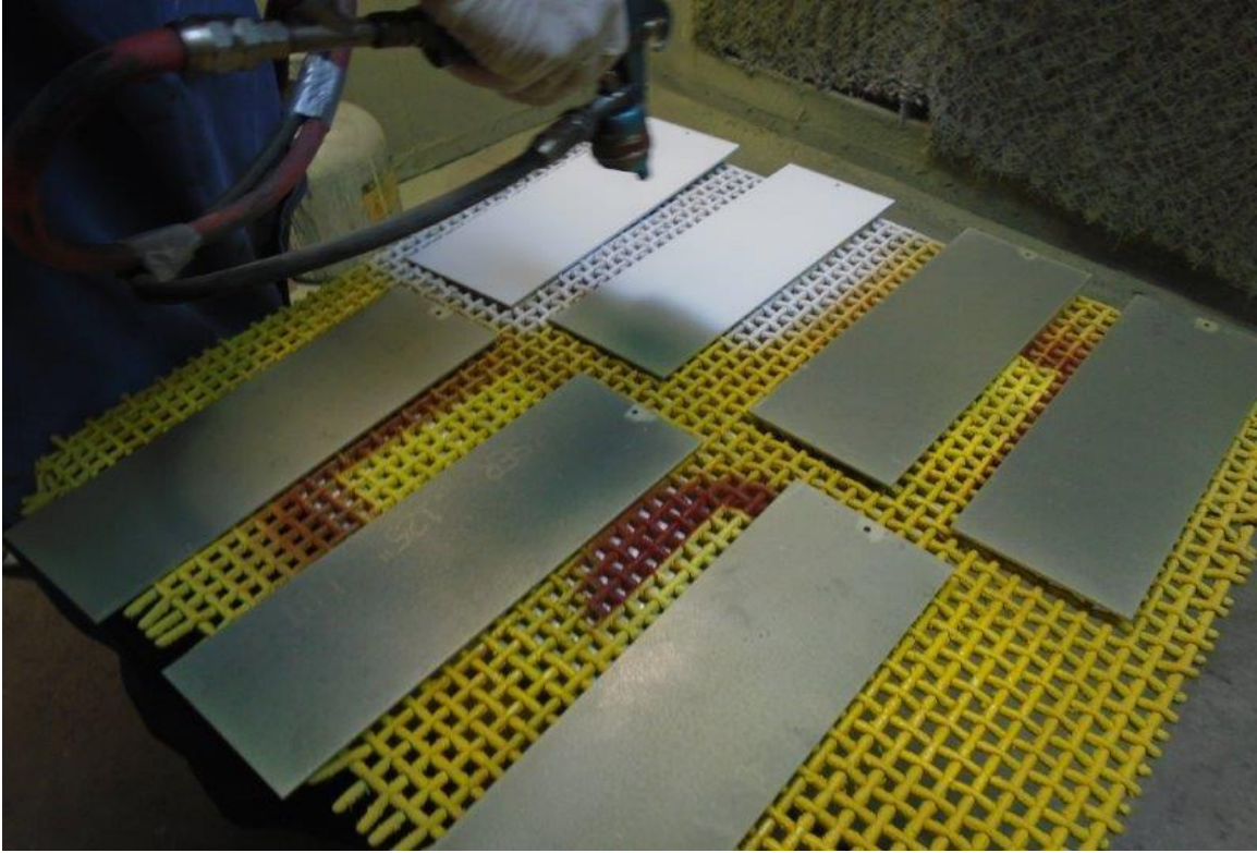
Figure 29. Coupons Coated with SILSBOND 01 (2%) Pretreatment coating
