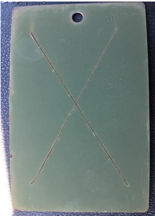
Figure 100. SILSBOND Pretreatment 01 (2%) + Primer + Topcoat on blasted CRS at 15 months
