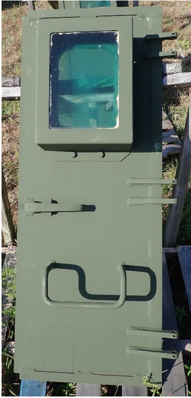
Figure 108. 3 Months Exposure Time for Bonderite M-NT 7400 Coating on Army MRAP Vehicle Door
