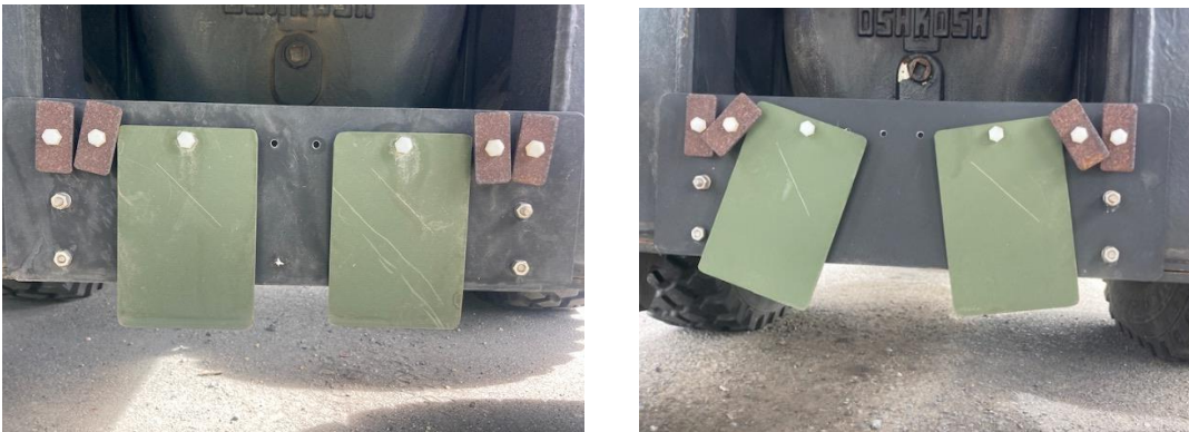
Figure 129. NSWCCD 12 Month Exposure Testing of SILSBOND 01 (2%) Pretreatment in Military Coating Stack-up on 1020 Steel Coupons
