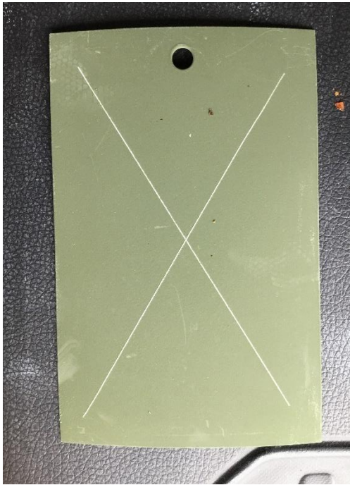
Figure 85. SILSBOND Pretreatment 01 (2%) + Primer + Topcoat on Blasted Al 2024-T3 at 18 months
