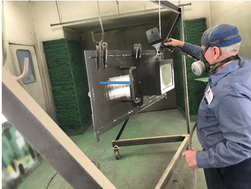
Figure 104. SILSBOND 01 (2%) Pretreatment Coating Application on MRAP Door Panel
