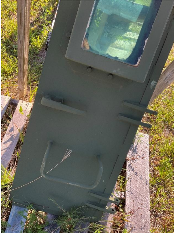
Figure 112. 15 Months Exposure Time for Bonderite M-NT 7400 Coating on Army MRAP Vehicle Door
