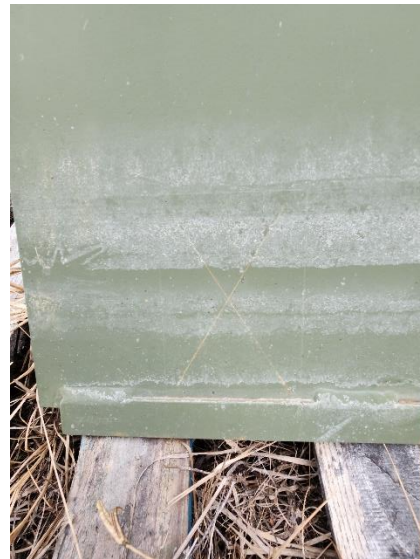
Figure 114. 24 Months Exposure Time for Bonderite M-NT 7400 Coating on Army MRAP Vehicle Door
