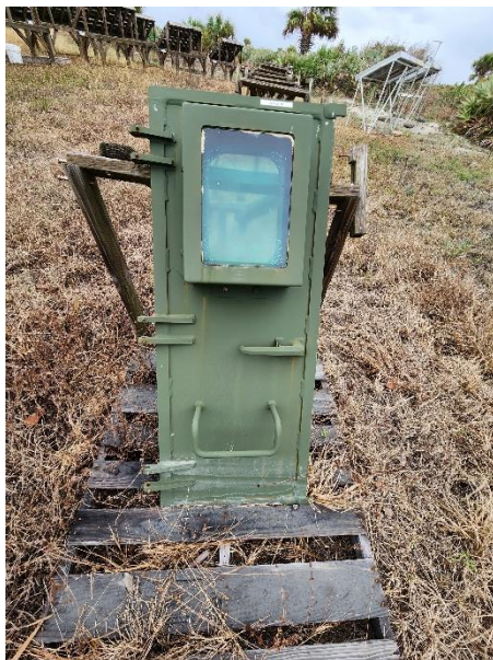
Figure 121. 24 Month Exposure Time for SILSBOND 01 (2%) Pretreatment Coating on Army MRAP Vehicle Door
