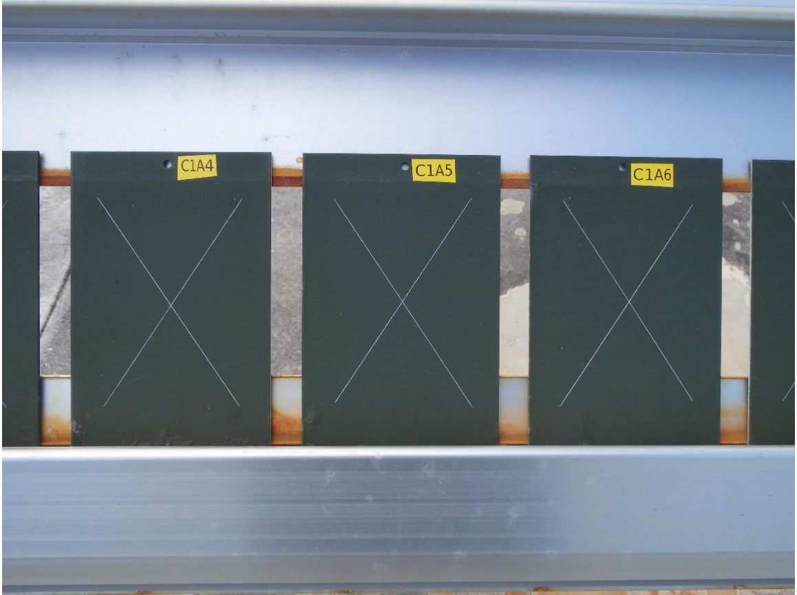
Figure 61. SILSBOND 01 (2%) on Al 2024-T3 at 0 Months
