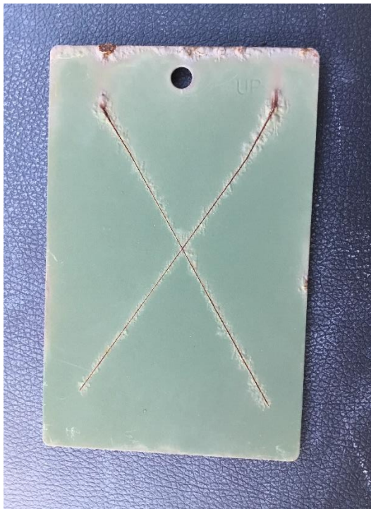
Figure 92. SILSBOND Pretreatment 01 (2%) + Primer + Topcoat on mil finished CRS at 15 months
