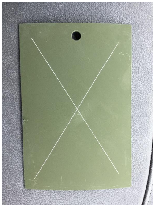
Figure 86. SILSBOND Pretreatment 01 (2%) + Primer + Topcoat on Blasted Al 2024-T3 at 24 months
