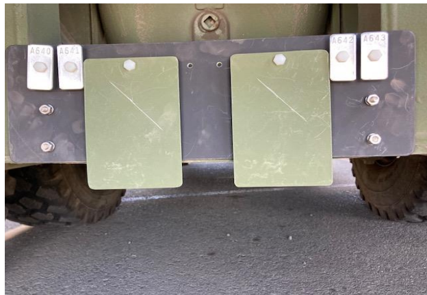
Figure 123. NSWCCD 3 Months Exposure Testing of SILSBOND 01 (2%) Pretreatment Coating in Military Coating Stack-up on 1020 Steel Coupons
