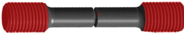
Figure 16. ASTM F-519 Hydrogen embrittlement specimen
