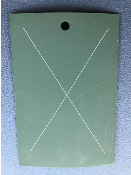
Figure 82. SILSBOND Pretreatment 01 (2%) + Primer + Topcoat on Blasted Al 2024-T3 at 9 months
