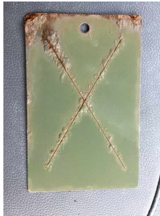
Figure 94. SILSBOND Pretreatment 01 (2%) + Primer + Topcoat on mil finished CRS at 24 months
