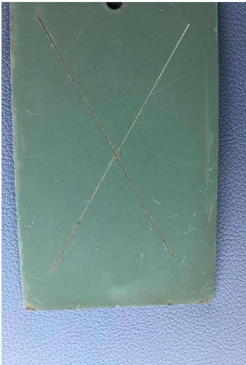
Figure 98. SILSBOND Pretreatment 01 (2%) + Primer + Topcoat on blasted CRS at 9 months
