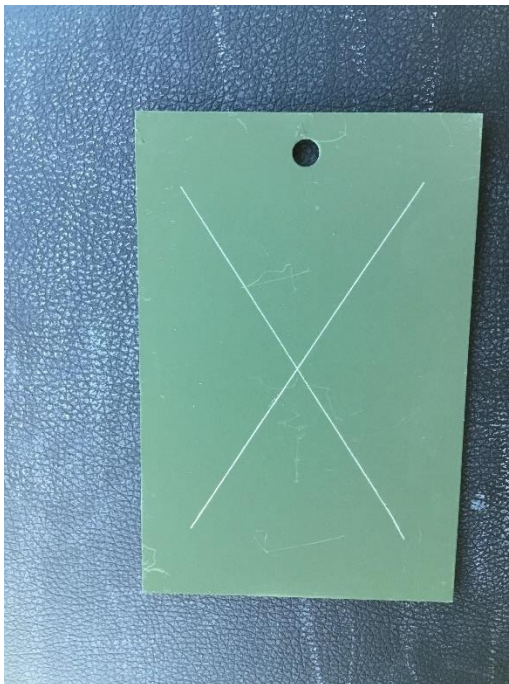
Figure 76. SILSBOND Pretreatment 01 (2%) + Primer + Topcoat on mil finished Al 2024-T3 at 15 months
