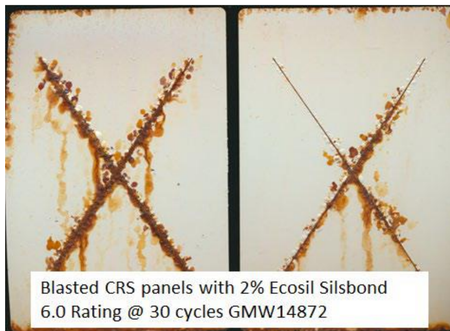
Figure 50. ARL Cyclic Corrosion Testing 1020 Steel with Rating of 6.0
