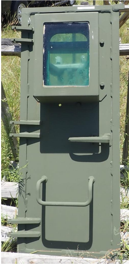
Figure 116. 6 Month Exposure Time for SILSBOND 01 (2%) Pretreatment Coating on Army MRAP Vehicle Door
