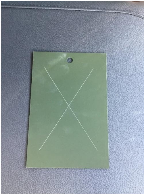
Figure 75. SILSBOND Pretreatment 01 (2%) + Primer + Topcoat on mil finished Al 2024-T3 at 12 months
