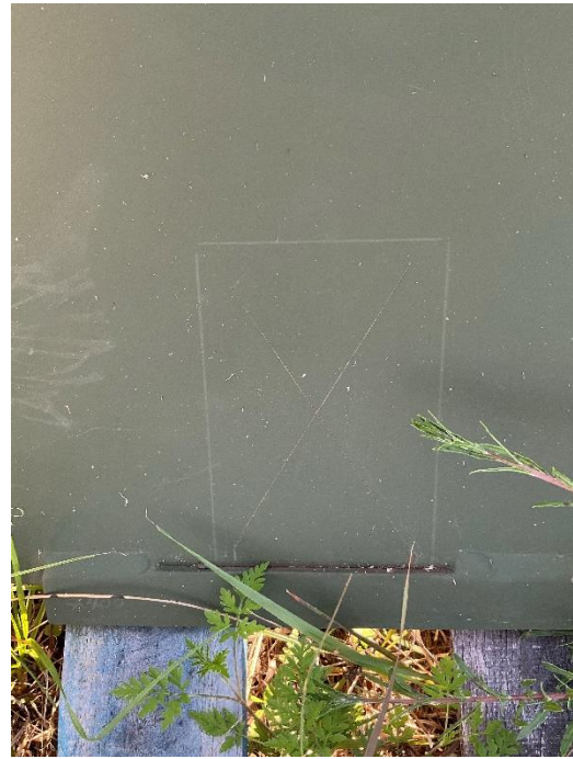
Figure 112. 15 Months Exposure Time for Bonderite M-NT 7400 Coating on Army MRAP Vehicle Door
