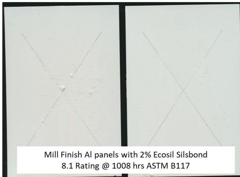
Figure 48. ARL NSS Testing Passing Criteria for Al 2024-T3 >8, no blisters >1mm
