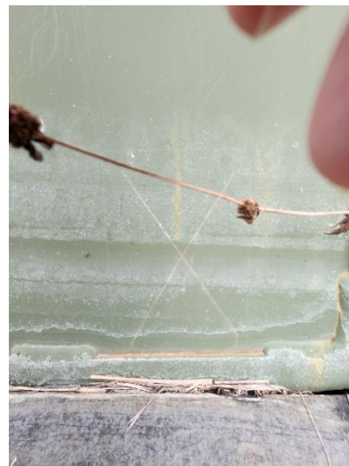
Figure 121. 24 Month Exposure Time for SILSBOND 01 (2%) Pretreatment Coating on Army MRAP Vehicle Door
