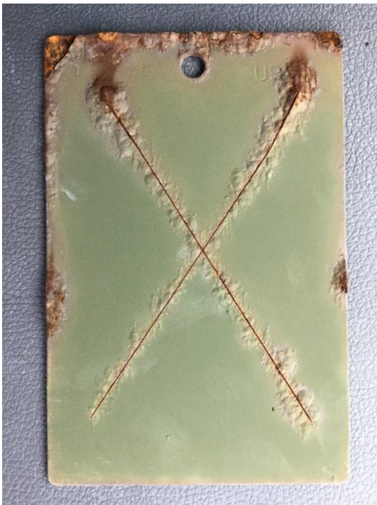
Figure 94. SILSBOND Pretreatment 01 (2%) + Primer + Topcoat on mil finished CRS at 24 months
