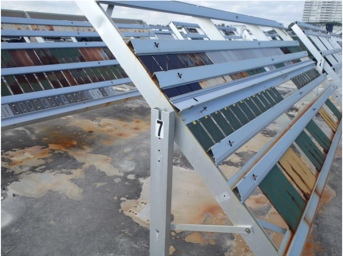
Figure 57. Racks Holding SILSBOND Pretreatment 01 (2%) + Primer + Topcoat at 24 Months
