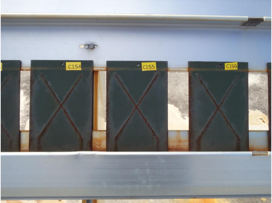
Figure 69. SILSBOND 01 (2%) coating on 1020 Steel at 12 Months
