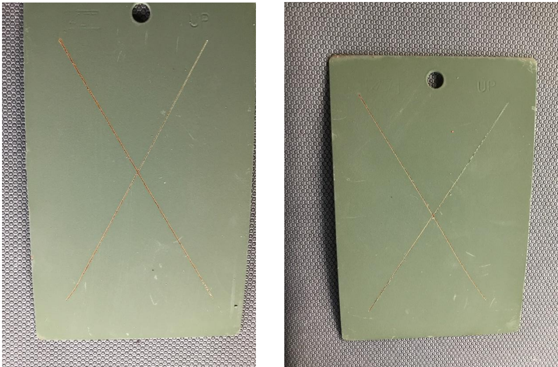
Figure 96. SILSBOND Pretreatment 01 (2%) + Primer + Topcoat on blasted CRS at 3 months
