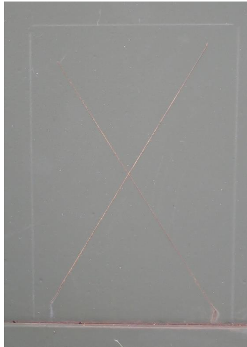
Figure 111. 12 Months Exposure Time for Bonderite M-NT 7400 Coating on Army MRAP Vehicle Door
