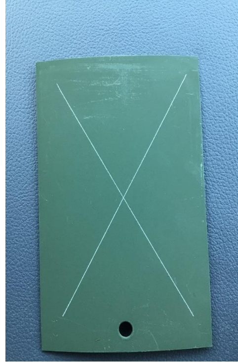
Figure 82. SILSBOND Pretreatment 01 (2%) + Primer + Topcoat on Blasted Al 2024-T3 at 9 months
