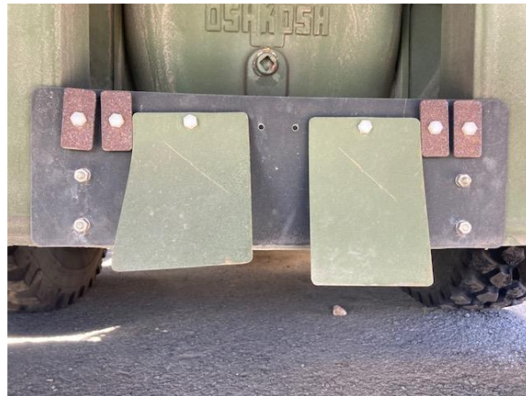
Figure 127. NSWCCD 9 Month Exposure Testing of SILDSBOND 01 (2%) Pretreatment Coating in Military Coating Stack-up on 1020 Steel Coupons
