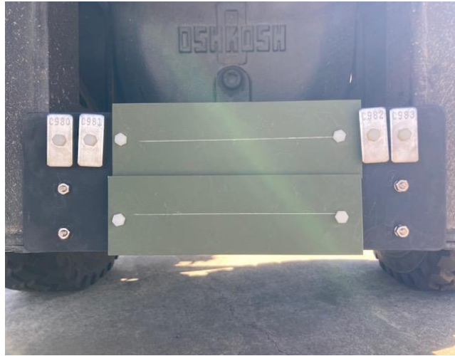
Figure 122. NSWCCD 3 Month Exposure Time of SILSBOND 01 (2%) Pretreatment in Military Coating Stack-up on Al 2024-T3 Coupons.
