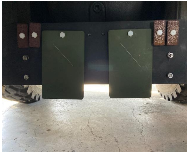
Figure 125. NSWCCD 6 Months Exposure Testing of SILDSBOND 01 (2%) Pretreatment Coating in Military Coating Stack-up on 1020 Steel Coupons
