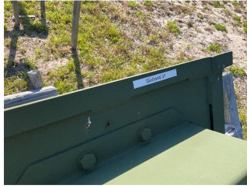
Figure 119. 15 Month Exposure Time for SILSBOND 01 (2%) Pretreatment Coating on Army MRAP Vehicle Door
