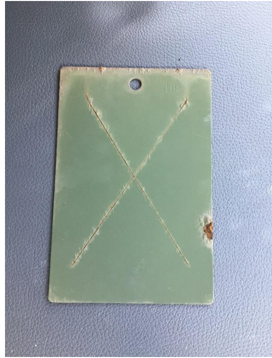
Figure 91. SILSBOND Pretreatment 01 (2%) + Primer + Topcoat on mil finished CRS at 12 months
