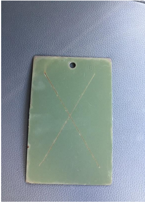
Figure 99. SILSBOND Pretreatment 01 (2%) + Primer + Topcoat on blasted CRS at 12 months
