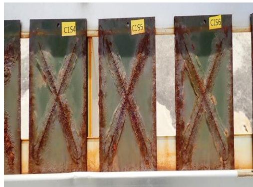
Steel coated with SILSBOND 01 (1.5%) (Steel 1020, MIL-DTL-53022 TIV/ MIL-DTL-53039)
