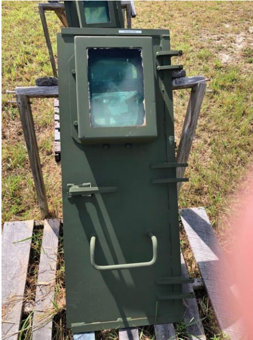
Figure 110. 9 Months Exposure Time for Bonderite M-NT 7400 Coating on Army MRAP Vehicle Door
