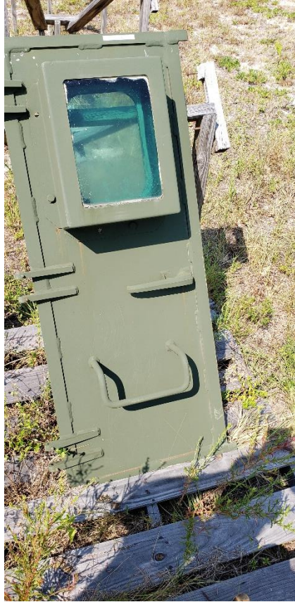
Figure 120. 18 Month Exposure Time for SILSBOND 01 (2%) Pretreatment Coating on Army MRAP Vehicle Door
