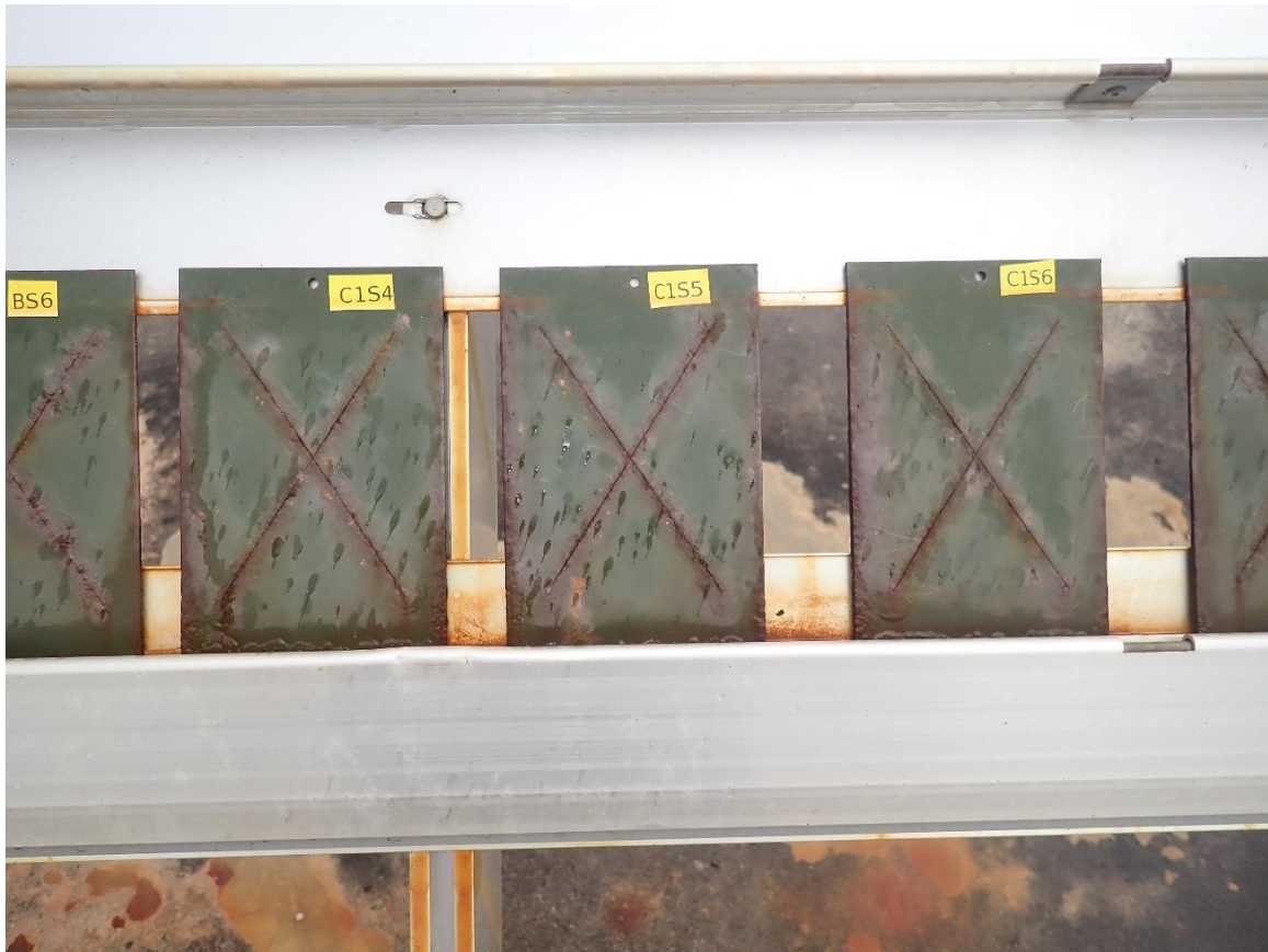
Figure 70. SILSBOND 01 (2%) on 1020 Steel at 24 Months
