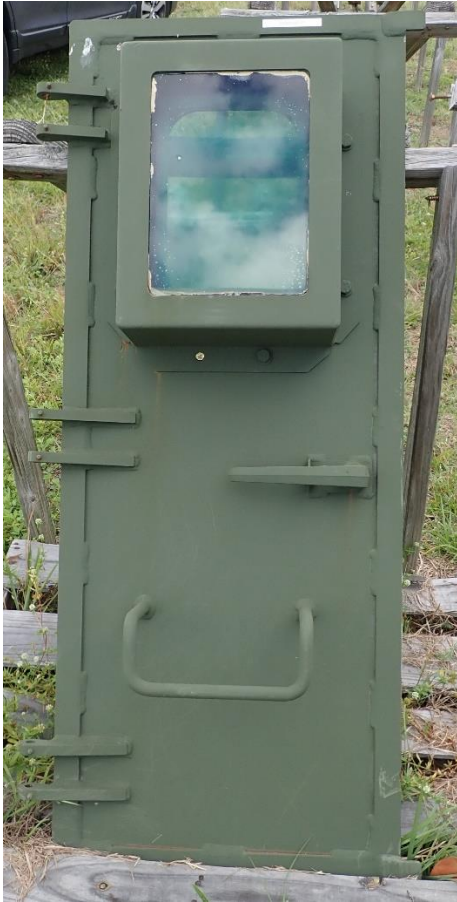
Figure 118. 12 Month Exposure Time for SILSBOND 01 (2%) Pretreatment Coating on Army MRAP Vehicle Door
