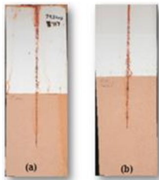
Figure 7. 800-hr NSS, CARC Painted HRS (a) SILBOND Pretreatment and (b) Zn/P Hexavalent Chromium Sealer
