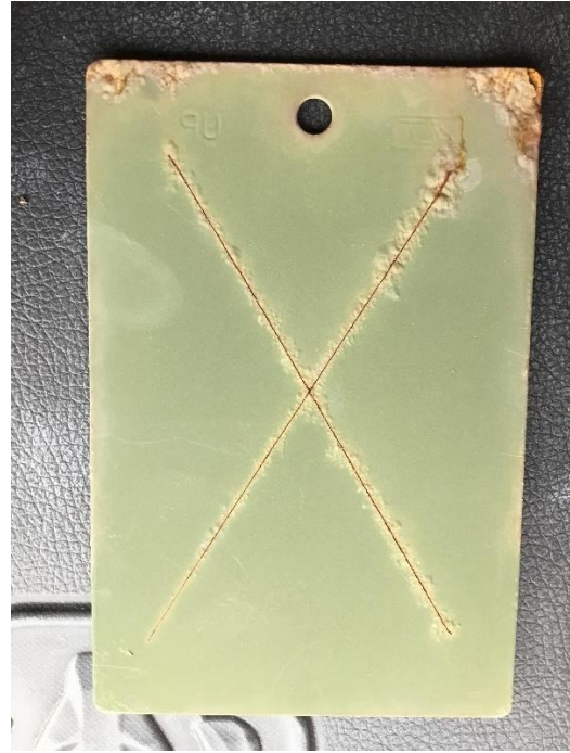
Figure 93. SILSBOND Pretreatment 01 (2%) + Primer + Topcoat on mil finished CRS at 18 months
