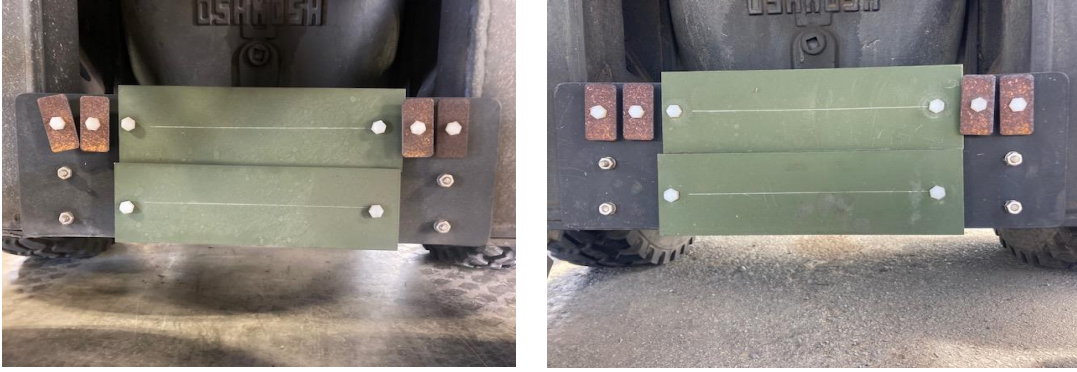
Figure 128. NSWCCD 12 Month Exposure Testing of SILSBOND 01 (2%) Pretreatment in Military Coating Stack-up on Al 2024-T3 Coupons
