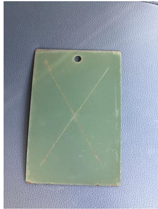
Figure 99. SILSBOND Pretreatment 01 (2%) + Primer + Topcoat on blasted CRS at 12 months
