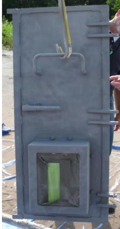
Figure 11. Freshly Abrasive Blasted MRAP Door Prior to the Application Pretreatment
