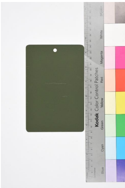
Figure 123. NSWCCD 3 Months Exposure Testing of SILSBOND 01 (2%) Pretreatment Coating in Military Coating Stack-up on 1020 Steel Coupons
