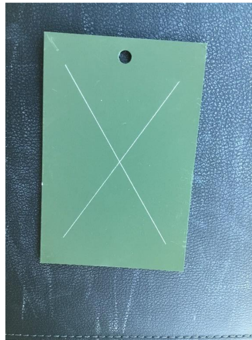
Figure 76. SILSBOND Pretreatment 01 (2%) + Primer + Topcoat on mil finished Al 2024-T3 at 15 months
