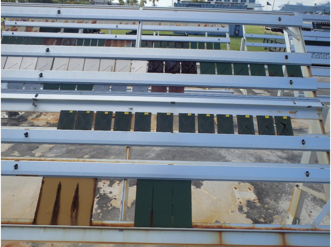
Figure 56. Racks holding SILSBOND Pretreatment 01 (2%) + Primer + Topcoat at 18 Months
