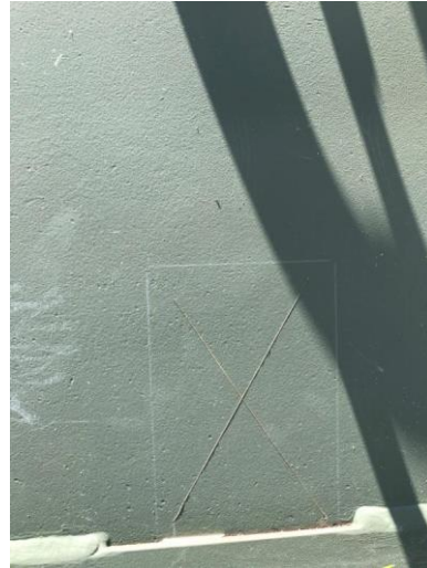
Figure 110. 9 Months Exposure Time for Bonderite M-NT 7400 Coating on Army MRAP Vehicle Door
