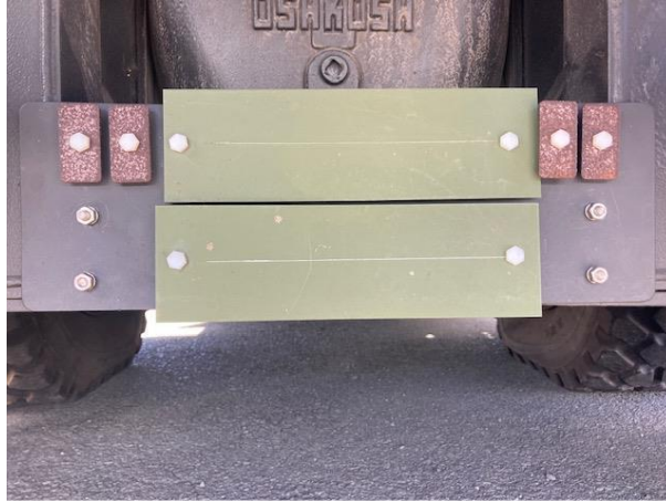
Figure 126. NSWCCD 9 Month Exposure Testing of SILDSBOND 01 (2%) Pretreatment Coating in Military Coating Stack-up on Al 2024-T3 Coupons
