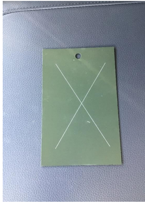
Figure 75. SILSBOND Pretreatment 01 (2%) + Primer + Topcoat on mil finished Al 2024-T3 at 12 months
