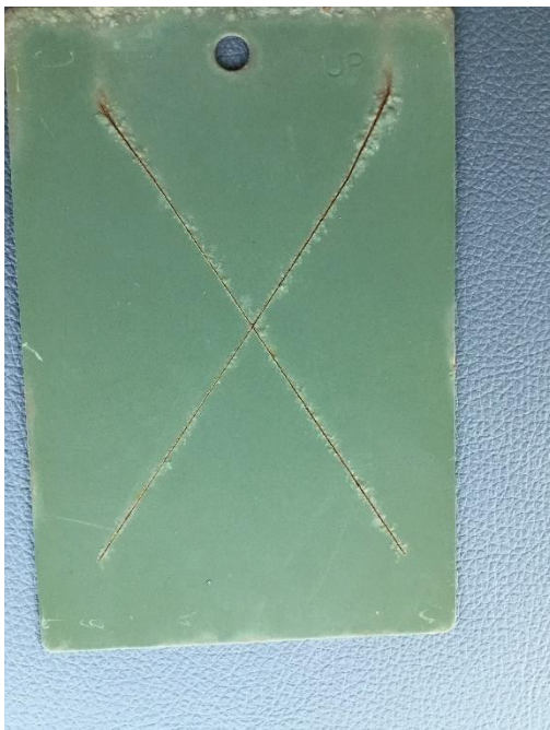
Figure 90. SILSBOND Pretreatment 01 (2%) + Primer + Topcoat on mil finished CRS at 9 months
