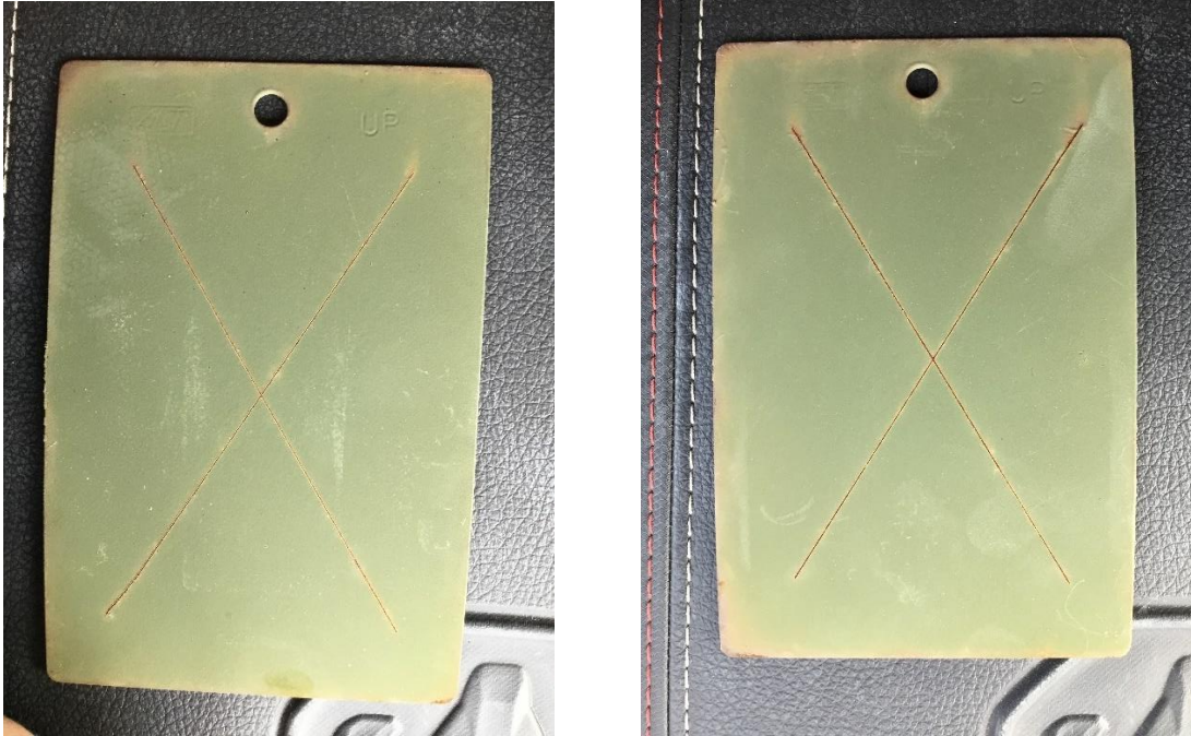
Figure 101. SILSBOND Pretreatment 01 (2%) + Primer + Topcoat on blasted CRS at 18 months
