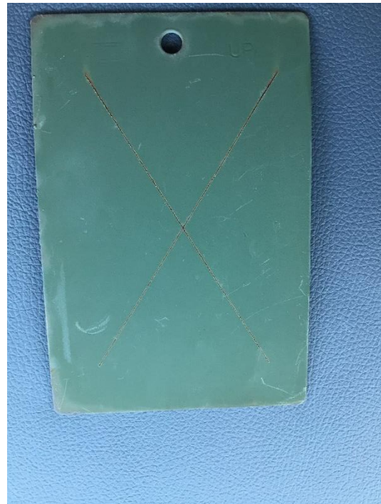
Figure 98. SILSBOND Pretreatment 01 (2%) + Primer + Topcoat on blasted CRS at 9 months
