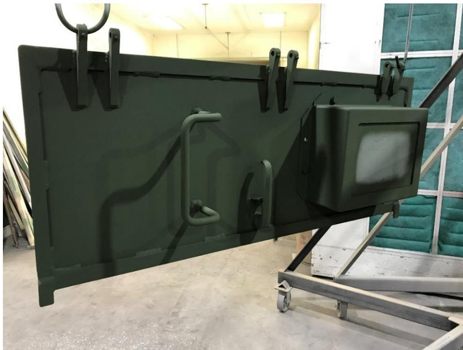
Figure 107. Full Military Coating w/SILSBOND 01 (2%) Pretreatment on Army MRAP Door Panel
