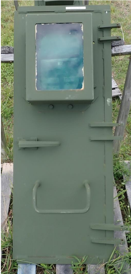
Figure 111. 12 Months Exposure Time for Bonderite M-NT 7400 Coating on Army MRAP Vehicle Door
