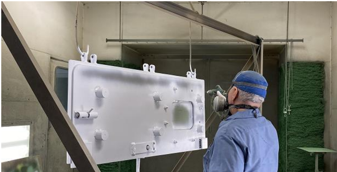
Figure 105. Epoxy priming of SILSBOND 01 (2%) Pretreatment Coating with MIL-DTL-53022TIV Epoxy Primer on Pretreated Door Panel
