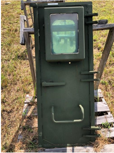
Figure 117. 9 Month Exposure Time for SILSBOND 01 (2%) Pretreatment Coating on Army MRAP Vehicle Door
