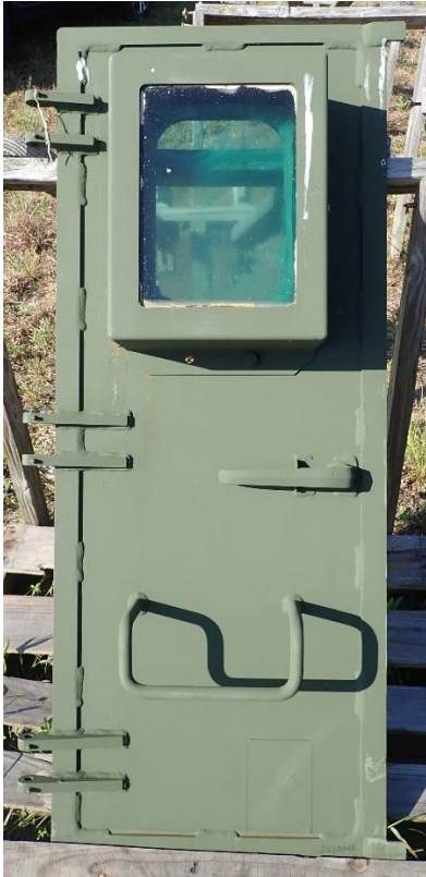
Figure 115. 3 Months Exposure Time for SILSBOND 01 (2%) Pretreatment Coating on Army MRAP Vehicle Door
