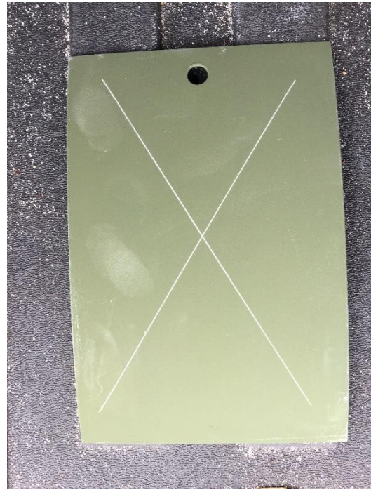
Figure 87. SILSBOND Pretreatment 01 (2%) + Primer + Topcoat on Blasted Al 2024-T3 at 27 months
