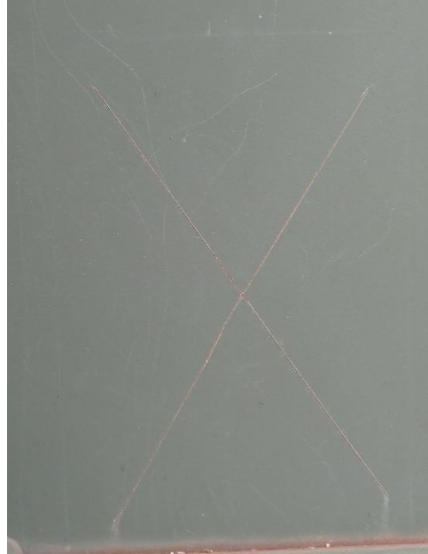
Figure 118. 12 Month Exposure Time for SILSBOND 01 (2%) Pretreatment Coating on Army MRAP Vehicle Door
