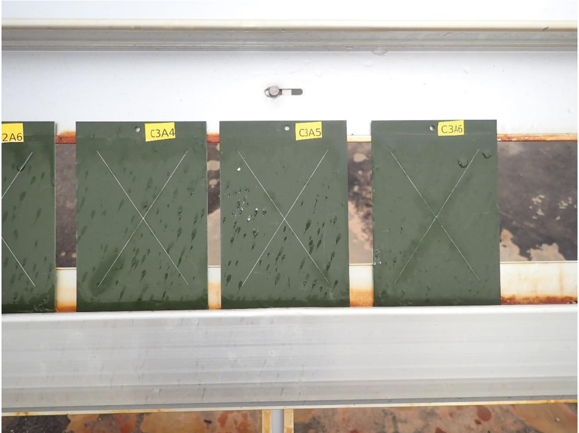
Figure 66. SILSBOND 05 (50%) on Al 2024-T3 at 24 Months
