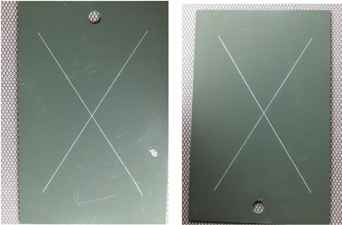
Figure 73. SILSBOND Pretreatment 01 (2%) + Primer + Topcoat on mil finished Al 2024-T3 at 6 months
