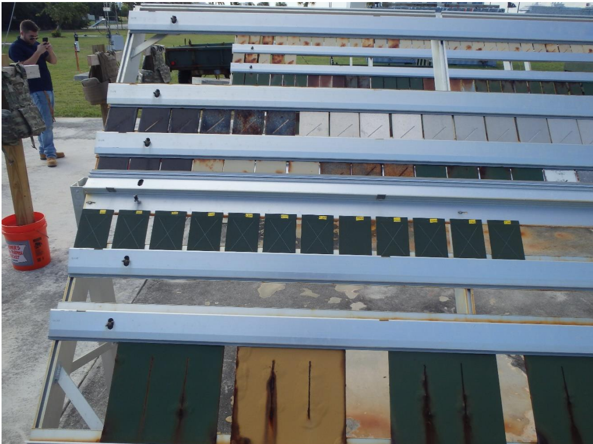
Figure 54. Racks Holding SILSBOND Pretreatment 01 (2%) + Primer + Topcoat at 0 months (location NSWCCD, Fort Lauderdale, FL marine outdoor corrosion testing site)
