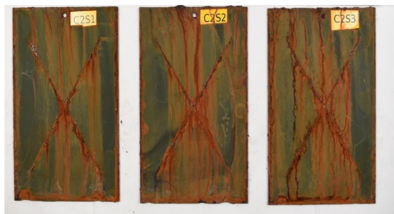
Figure 40. NSWCCD Round Robin Test Results SILSBOND 01 (3%) Coated 1020 Steel Panels
