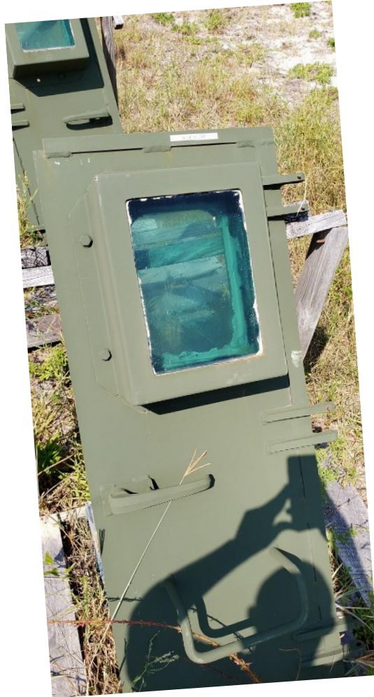
Figure 113. 18 Months Exposure Time for Bonderite M-NT 7400 Coating on Army MRAP Vehicle Door
