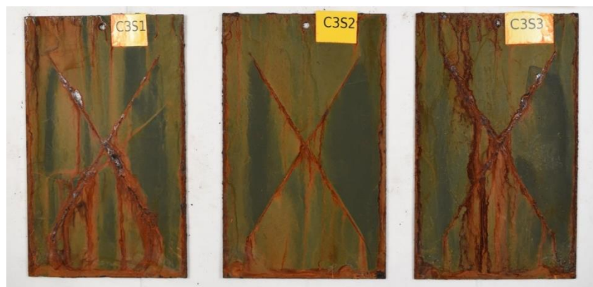
Figure 41. NSWCCD Round Robin Test Results SILSBOND 05 (50%) Coated 1020 Steel Panels
