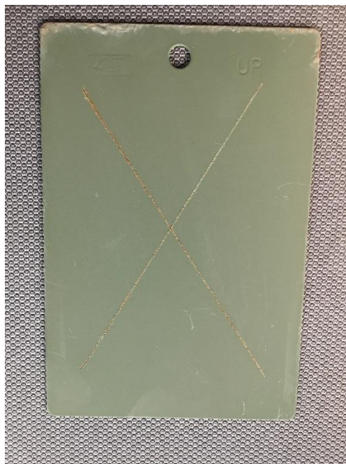
Figure 88. SILSBOND Pretreatment 01 (2%) + Primer + Topcoat on mil finished CRS at 3 months
