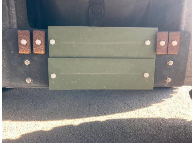
Figure 124. NSWCCD 6 Month Exposure Testing of SILDSBOND 01 (2%) Pretreatment Coating in Military Coating Stack-up on Al 2024-T3
