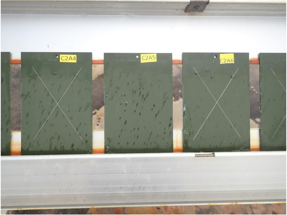
Figure 64. SILSBOND 01 (3%) on Al 2024-T3 at 24 Months
