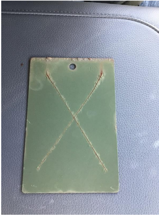
Figure 91. SILSBOND Pretreatment 01 (2%) + Primer + Topcoat on mil finished CRS at 12 months
