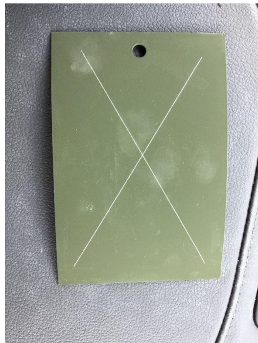
Figure 86. SILSBOND Pretreatment 01 (2%) + Primer + Topcoat on Blasted Al 2024-T3 at 24 months
