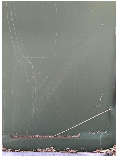
Figure 117. 9 Month Exposure Time for SILSBOND 01 (2%) Pretreatment Coating on Army MRAP Vehicle Door
