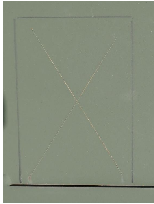
Figure 108. 3 Months Exposure Time for Bonderite M-NT 7400 Coating on Army MRAP Vehicle Door
