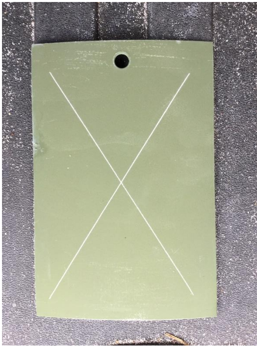
Figure 87. SILSBOND Pretreatment 01 (2%) + Primer + Topcoat on Blasted Al 2024-T3 at 27 months
