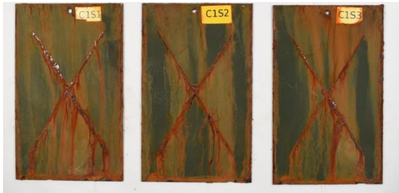
Figure 39. NSWCCD Round Robin Test Results SILSBOND 01 (1.5%) Coated 1020 Steel Panels
