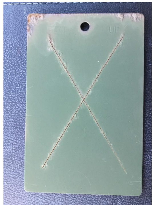
Figure 92. SILSBOND Pretreatment 01 (2%) + Primer + Topcoat on mil finished CRS at 15 months
