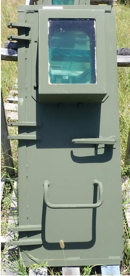
Figure 109. 6 Months Exposure Time for Bonderite M-NT 7400 Coating on Army MRAP Vehicle Door
