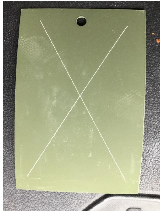
Figure 85. SILSBOND Pretreatment 01 (2%) + Primer + Topcoat on Blasted Al 2024-T3 at 18 months
