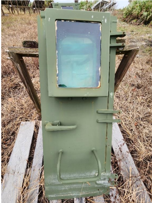
Figure 114. 24 Months Exposure Time for Bonderite M-NT 7400 Coating on Army MRAP Vehicle Door
