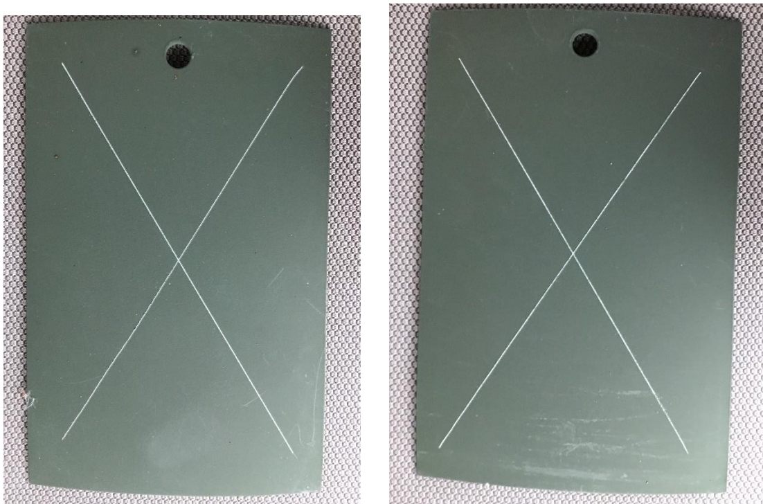
Figure 81. SILSBOND Pretreatment 01 (2%) + Primer + Topcoat on Blasted Al 2024-T3 at 6 months
