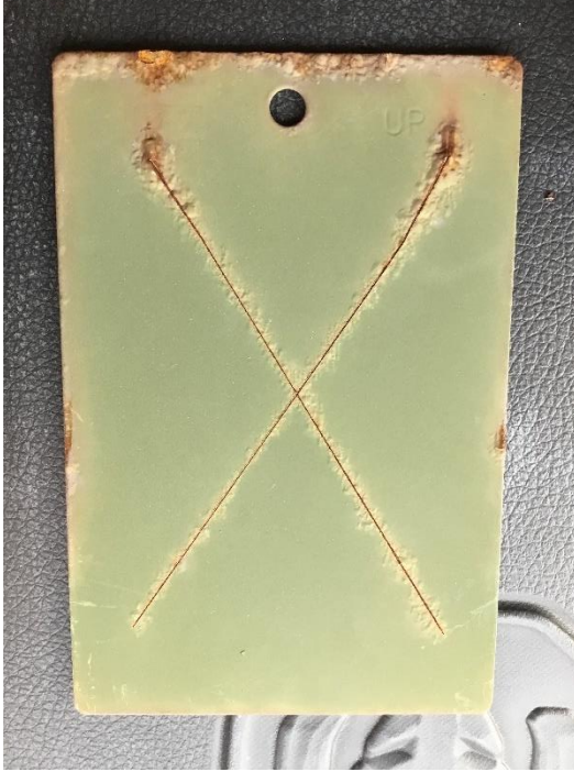
Figure 93. SILSBOND Pretreatment 01 (2%) + Primer + Topcoat on mil finished CRS at 18 months
