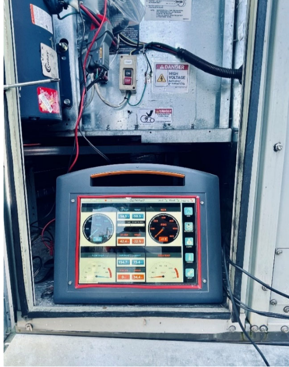
Figure ES-1. An i-Optimize Diagnostic Analyzer Being Used to Measure Performance of a Package AC Unit.
