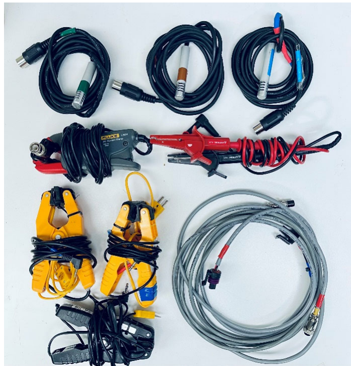
Figure ES-2. Clamps and Sensors Used with i-Optimize Diagnostic Analyzer.
