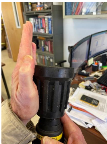
Fig. 4.4-2 – Finger Width Pattern Selection/Setting
