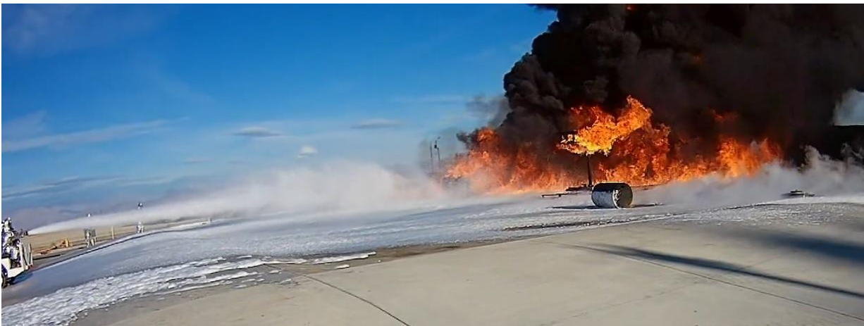
Fig. 4.5-2 – Horizontal Sweep Suppression Sequence
