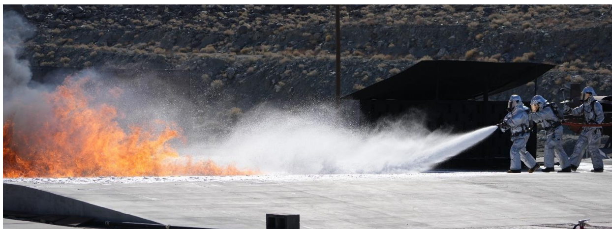
Fig. 4.5-4 – Roll-on Foam Application
