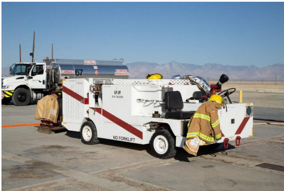
Fig. 3.4-6 – P-25A Shipboard Fire Truck (Photograph)
