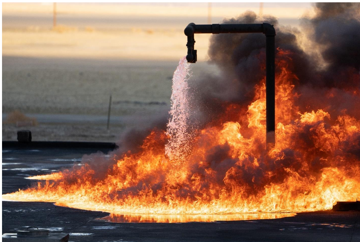
Fig. 4.6-1 – Flowing/Running Fuel Fire Scenario
