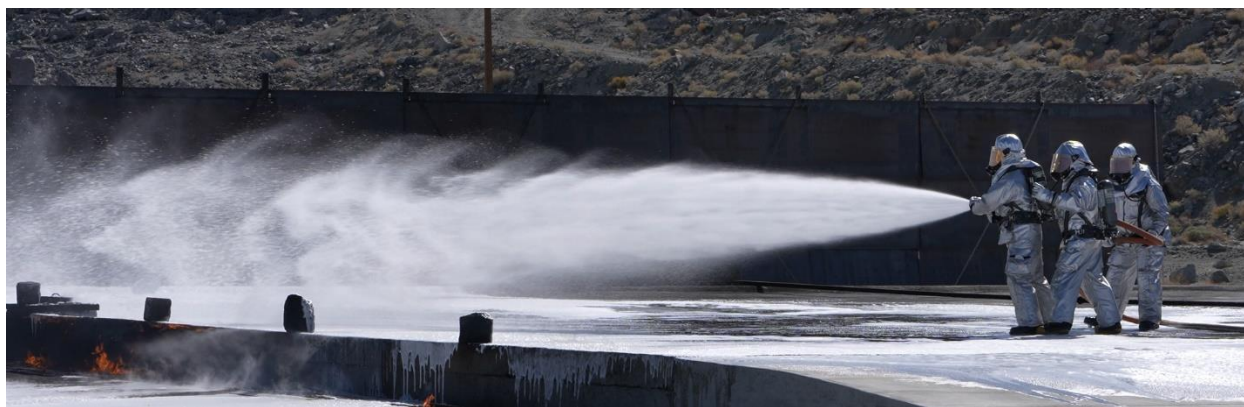
Fig. 4.4-3 – Slightly Wider Spray Pattern Used for Close-in Application
