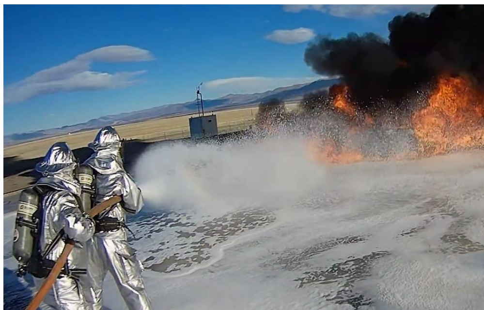
Fig. 4.5-3 – Rapid Foam Breakdown Shortly After Application
