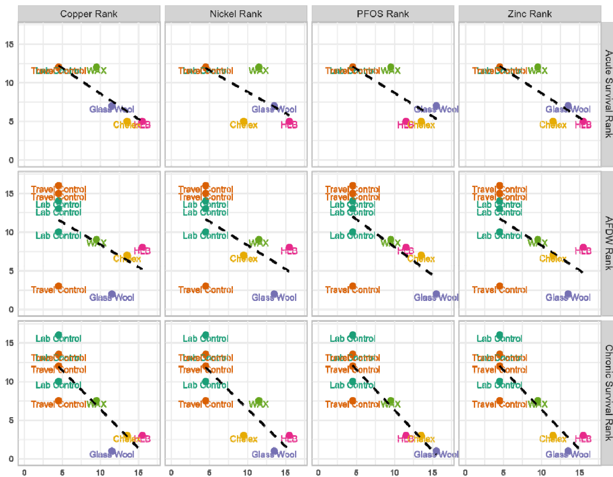
Figure 7.5.6: Plots depicting relationships between C. dilutus biological endpoints and chemistry data from Spearman's rank analyses for the iTIE experiments at the Rouge River. The dotted lines show correlation coefficients. Groups with lower ranks on the x-axis were exposed to lower concentrations of contaminants. Higher ranks for AFDW indicate higher mean weights of surviving organisms. Higher acute and chronic survival ranks indicate higher survival.
