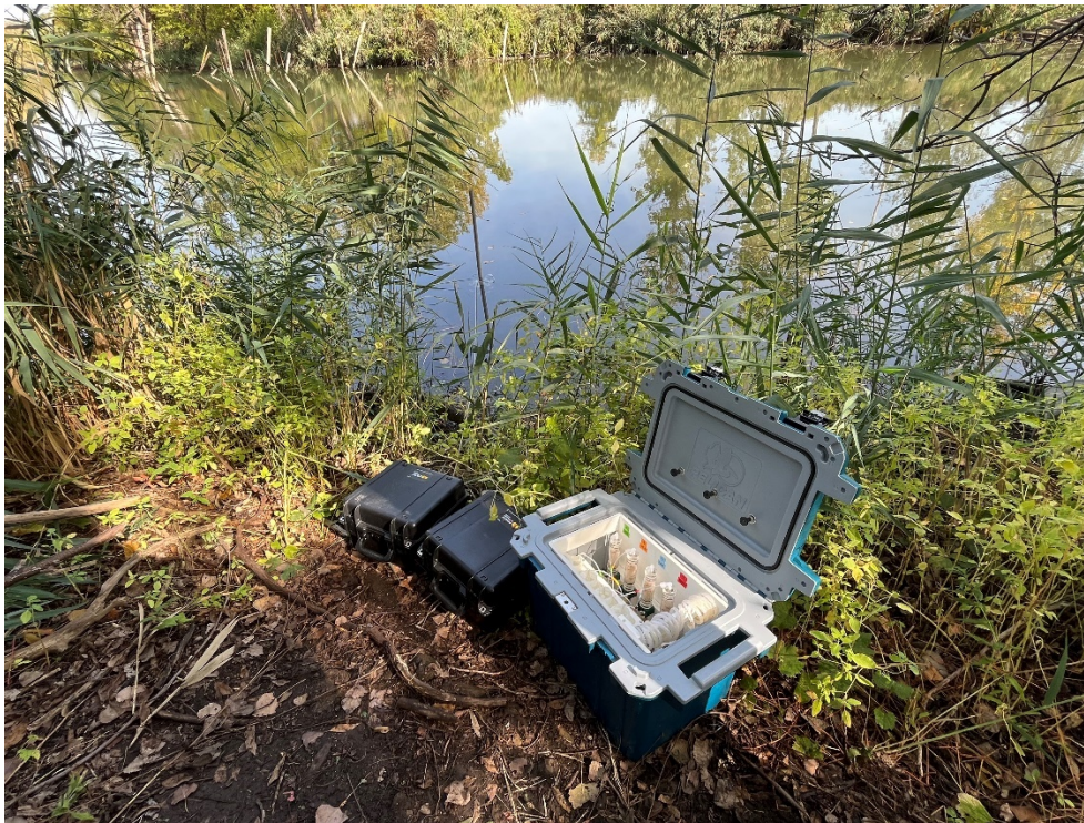
Figure 2.1.1: iTIES deployment at the Rouge River, Detroit, MI. In the foreground is the iTIE Cooler Sub-System, which contains iTIE resin treatments and test organism groups, as well as the oxygenation coil and sample collection bottles. Next to the iTIE Cooler are the two pump cases, which drive water movement through the entire system. The Trident can be seen above the pump cases, installed in the river channel near shore.
