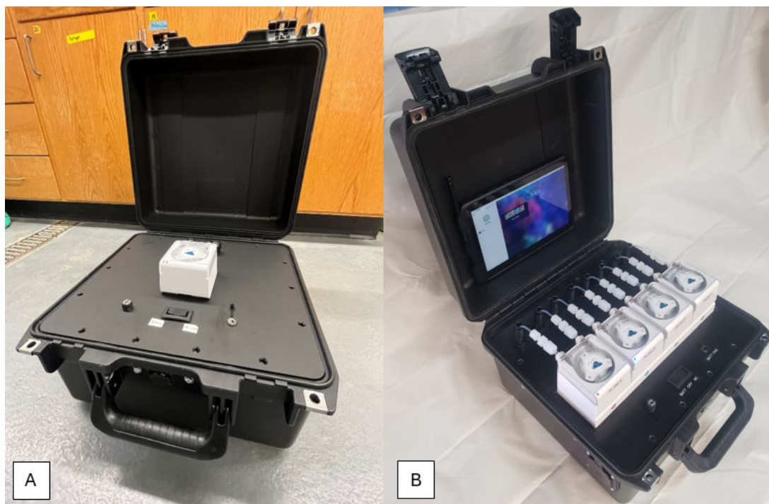
Figure 2.2.1: The iTIES Pumping Sub-System. A) The booster pump case, containing a single peristaltic pump. B) The quad pump case, containing four peristaltic pumps. A tablet is mounted inside the lid of the quad pump case, which can be used to program and operate both pump cases when connected to the internet.
