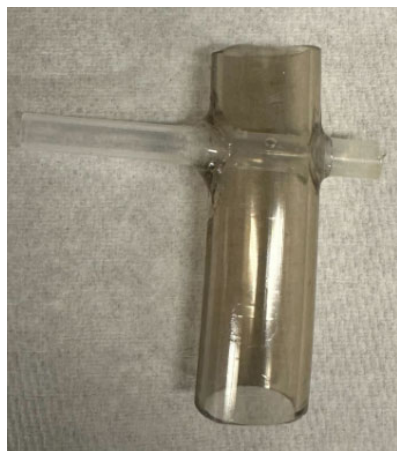
Figure 2.3.3: The iTIES drip chamber. This small chamber is oriented vertically, with the perpendicular tubing located near the top of the chamber. As water flows into the chamber, gas bubbles and excess water are sorted and diverted through the perpendicular tubing to an overflow collection bottle.
