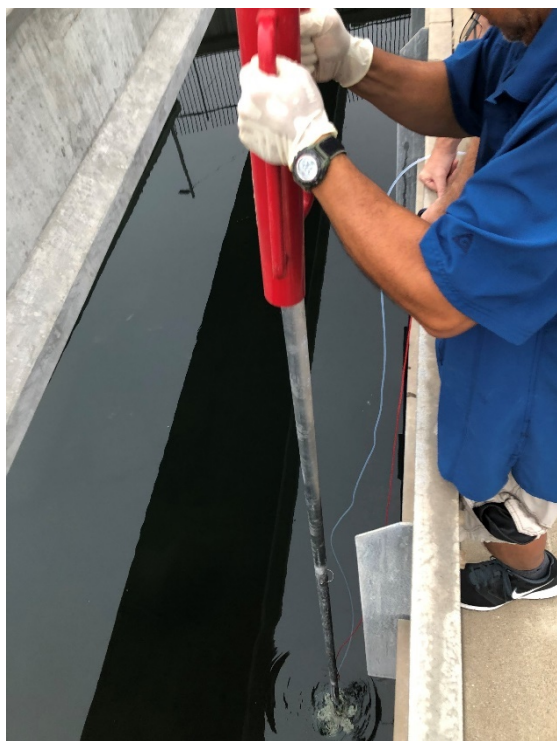
Figure 2.1.3: Trident probe installation. The Trident probe is installed using a series of push poles. After installation, these push poles can be disengaged and removed, leaving the Trident in place in the sediment. Tubing remains connected to the Trident, routing porewater to the iTIES. A rope is used to remove the Trident at the end of deployment.
