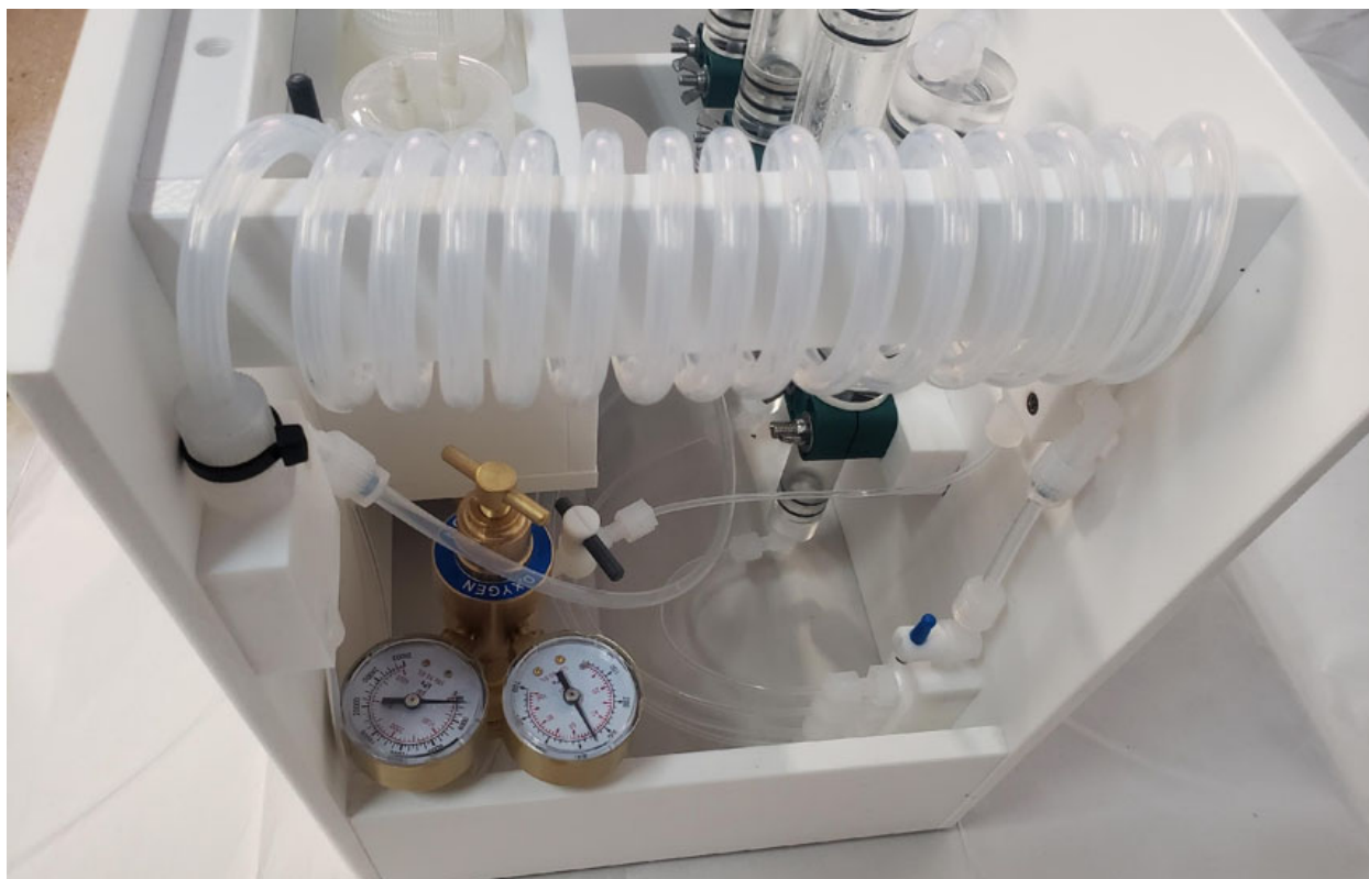
Figure 2.3.2: The iTIES oxygenation system. The oxygenation coil (top of picture) is built from nested tubing. The interior tubing of the coil is gas-permeable and pressurized with oxygen, which is supplied by an oxygen canister (hidden) that is controlled by a gas regulator (bottom left). Sampled water is exposed to the pressurized tubing as it flows through the exterior tubing.
