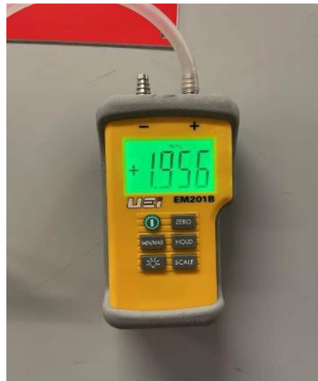
Figure 2-13. Handheld Digital Manometer for Measuring Duct Static Pressures
