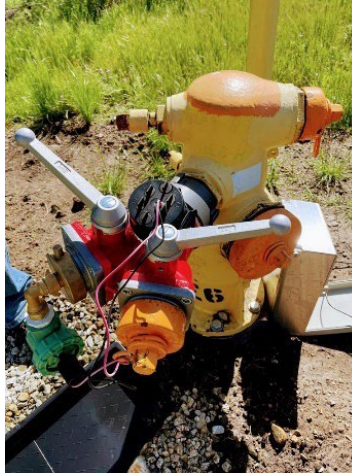
Figure ES-6. An Apparatus Attached to a Hydrant for Automating the Leak Flow.
