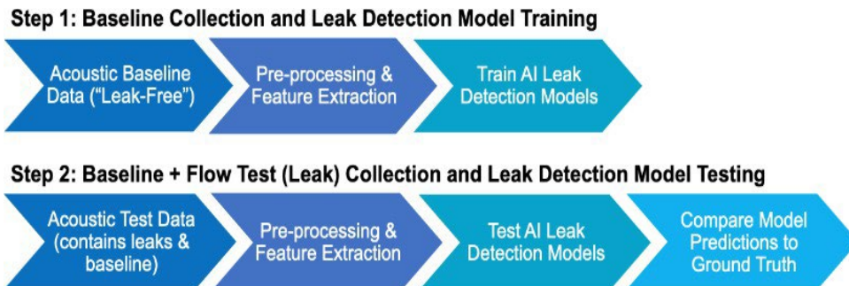
Figure ES-10. Overview of Baseline Learning & Leak Detection Model Testing Procedure.
