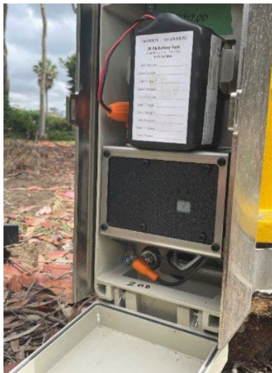
Figure ES-7. hydrant.AI Sensor Backhaul with a Wireless Communication Module for Phase-II.
