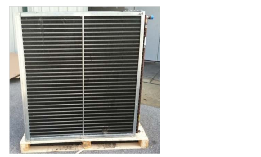
Figure 10. Large PCM-Filled Coil Prior to Installation at the Demonstration Site
