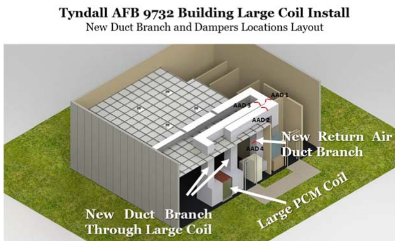
Figure 11. New Duct System after Integrating the Large PCM-Filled Coil
