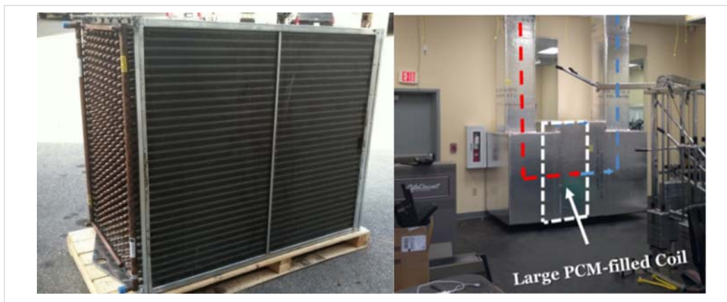
Figure 3. Large PCM-Filled Coil Unit
