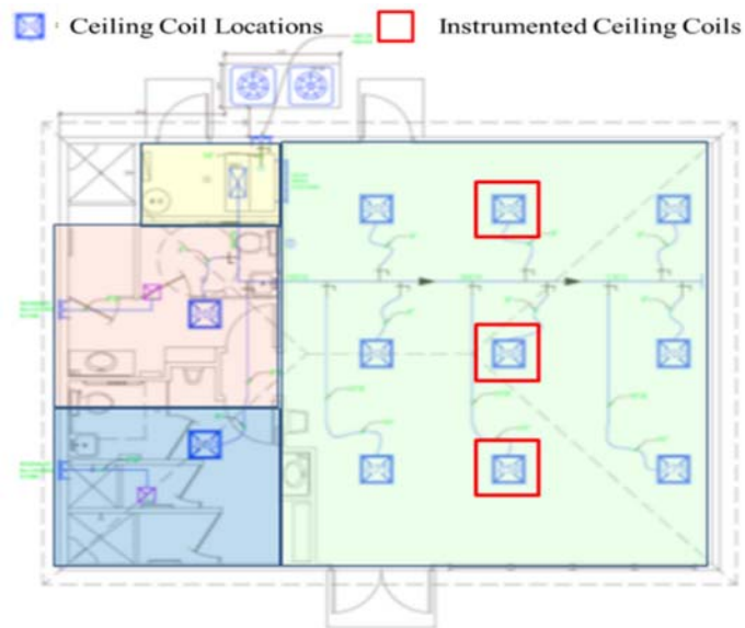
Figure 12. Instrumented Ceiling Coil Locations in the Demonstration Building
