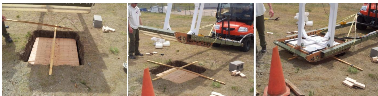
Figure 19. We carefully aligned a set of crosshairs with the center of the test grid (left) and then manually guided the MetalMapper sensor head (center, right).
