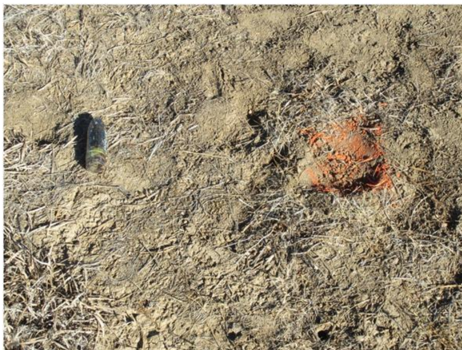
Figure 32. The actual target (37 mm) and the initial target pick coordinates (orange mark) corresponding to the survey described in the last several figures.
