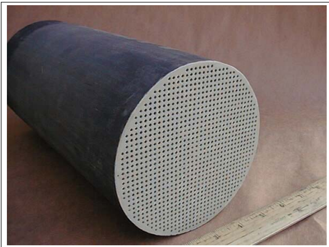
Figure 5. Full Size Filter (5.66" diameter x 12" length, 20 ft 2 area)
