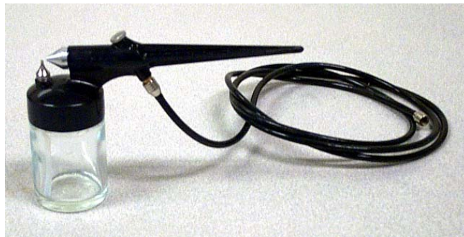
Figure 9: Device used for spray coating SABC on small scale test samples—Badger Model 250, single-action, external-mix, siphon-feed airbrush.
